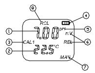
1. Main display - 31/2 digit display providing direct readout of pH or mV. Underrange (-1) and Overrange (1) symbols will be displayed if the instrument is reading outside the ranges of:
